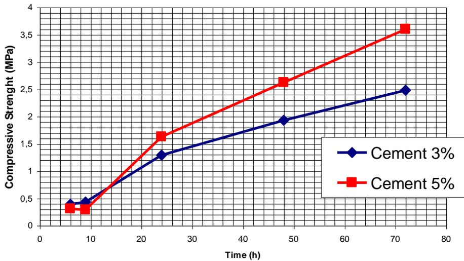
Figure 7. Effect of curing time on the compressive strength.
