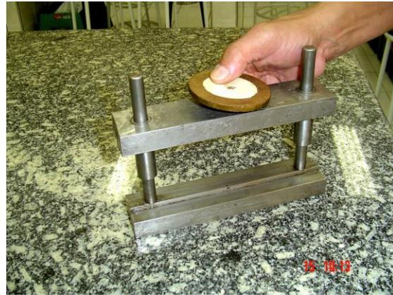
Figure 5: Some details of the Indirect Tensile Stress Apparatus
