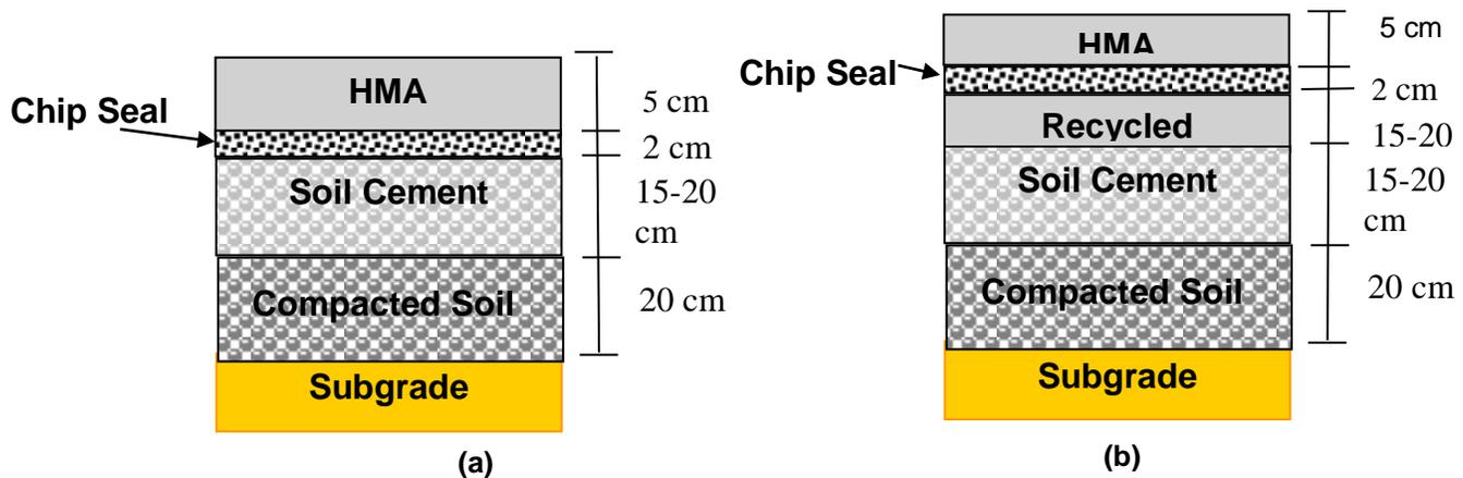
Figure 1 Typical Structure (a) before recycling (b) recycled in São Paulo State.
