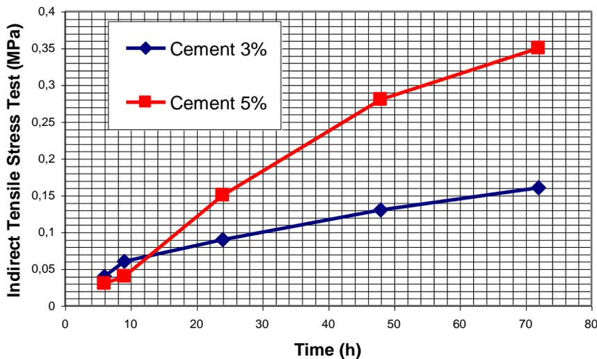
Figure 8. Effect of curing time on the indirect tensile stress.
