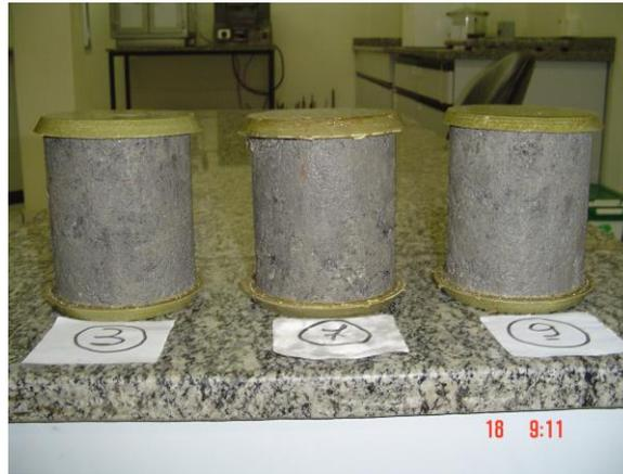
Figure 3: The capped specimens.
