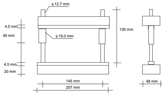
Figure 4: Apparatus used in Indirect Tensile Stress
