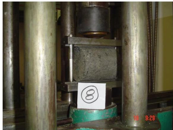
Figure 6: Indirect tensile stress test.
